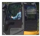
Raised operator cab (for special applications)
